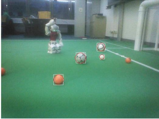
Figure III.1. The result of the ball detection as seen in the HULKs debug tool. Clustered regions are highlighted white, detected balls are circled red. Note, that the 2016 ball candidate is detected.
