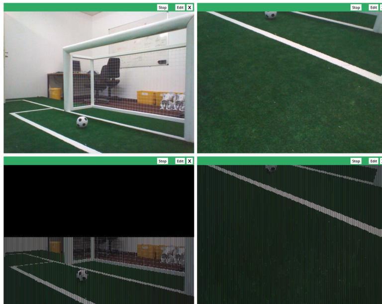
**Figure 3.1:** *The result of the image segmenter in the HULKs Framework. Top Left: The raw image from the upper camera. Top Right: The raw image from the lower camera. Bottom Left: The segmented image of the upper camera. Bottom Right: The segmented image of the lower camera. Areas above the horizon determined by the projected distance are ignored.*
