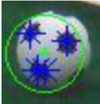
**Figure 3.3:** *Candidate (green circle with green cross in center) derived from merged seeds. The seeds (blue crosses) got merged as they are within the distance of the balls diameter. The candidates center and radius are determined by the mean of the projected radii and centers of the seeds.*
