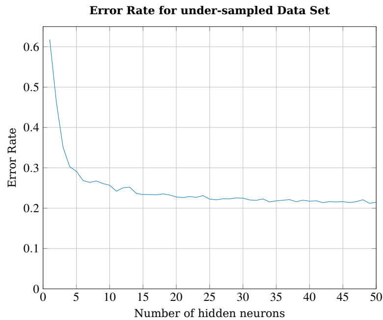
Figure 4.7: The Mean squared Error for a neural network with one hidden layer dependent on the number of neurons for the under-sampled data set.
