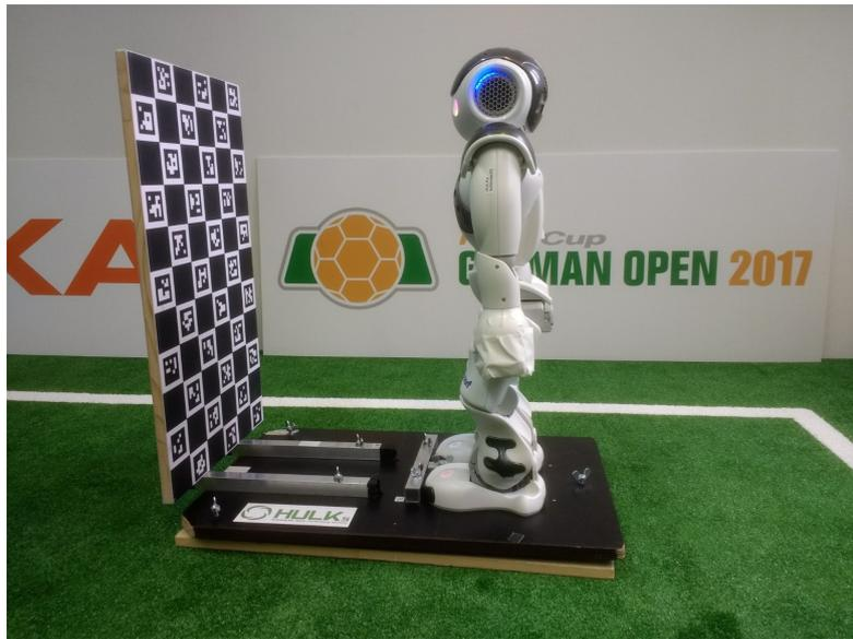
**Figure 3.3:** A NAO robot on calibration stand developed by HULKs for camera intrinsic and extrinsic calibration. It can also be used for joint calibration if necessary, but the proximity of calibration pattern seems to amplify any small amount of positioning errors of the robot.
