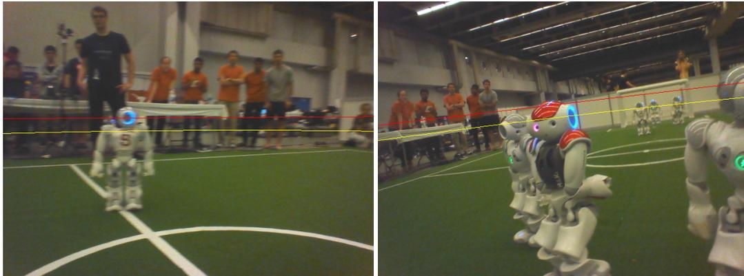
**Figure 3.6:** Two test images taken with the NAO’s top camera recorded at the RoboCup 2018 with the horizon marked by a red line. A yellow line marks the distance of 13 meters from the robots feet which is equivalent to the length of the field’s diagonal.
